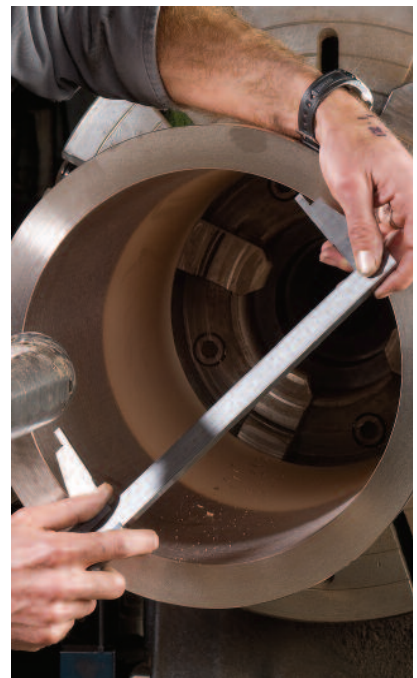
Centrifugal castings can be supplied machined to near net size.
