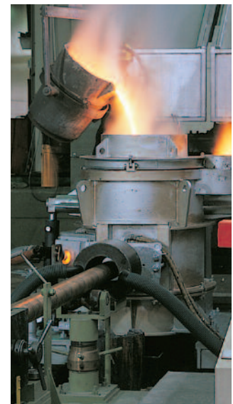
Roller indexing continuous casting line and furnace.
